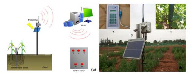
Figure 1. Long range telemetry system design (a), soil moisture sensor (b1), Data logger (b2) and soil moisture data transmitter (b3) used in the experiment of irrigation treatments of quinoa (*Chenopodium quinoa* Willd.) at Agadir, Morocco.
